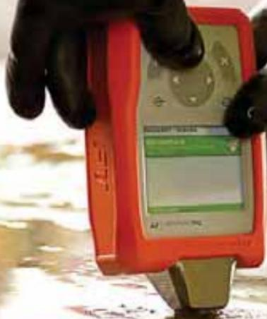
From the makers of FirstDefender, the revolutionary TruDefender™ FT handheld FTIR system enables identification of an even broader range of unknown chemicals—right in the hotzone.
