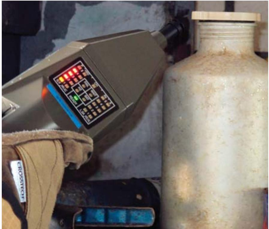
*QFES scientific officer inspecting canister found to contain aluminium phosphide with AP4C. The instrument display is showing a strong response to phosphorous ©QFES*
