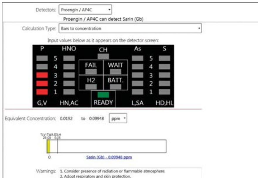
Emergency Response Decision Support System output for 3 bars on phosphorous channel of AP4C relative to Sarin ©QFES
