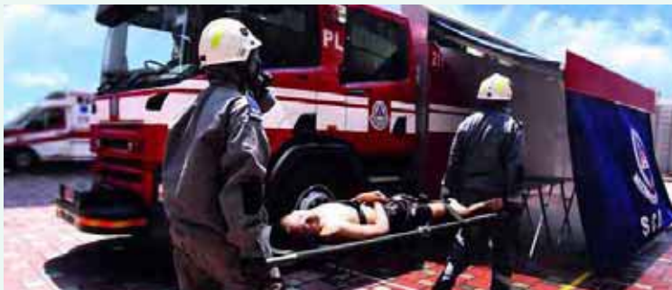
To enhance the decontamination capabilities of SCDF, fire engines have been retrofitted with the necessary accessories like shower heads and canopy to enable decontamination of casualties in a CBRN incident ©SCDF
