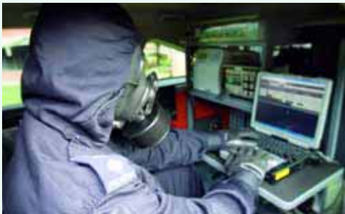
The HCV is equipped with a computer-aided zone modeling software mounted within the vehicle. ©SCDF
