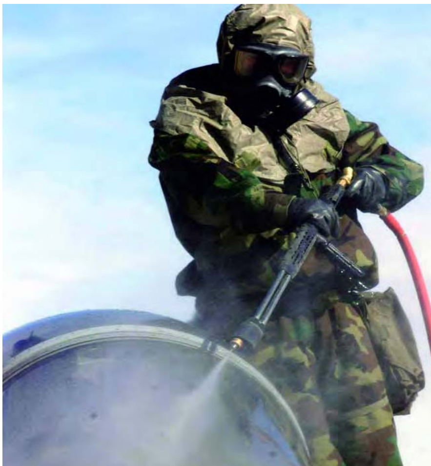
High pressure cleaning is not always the best policy for aircraft surfaces ©DoD
