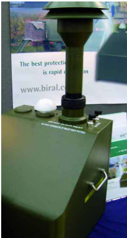
Biral's Verotect is the biological detector for the UK's ISMS ©CBRN World
